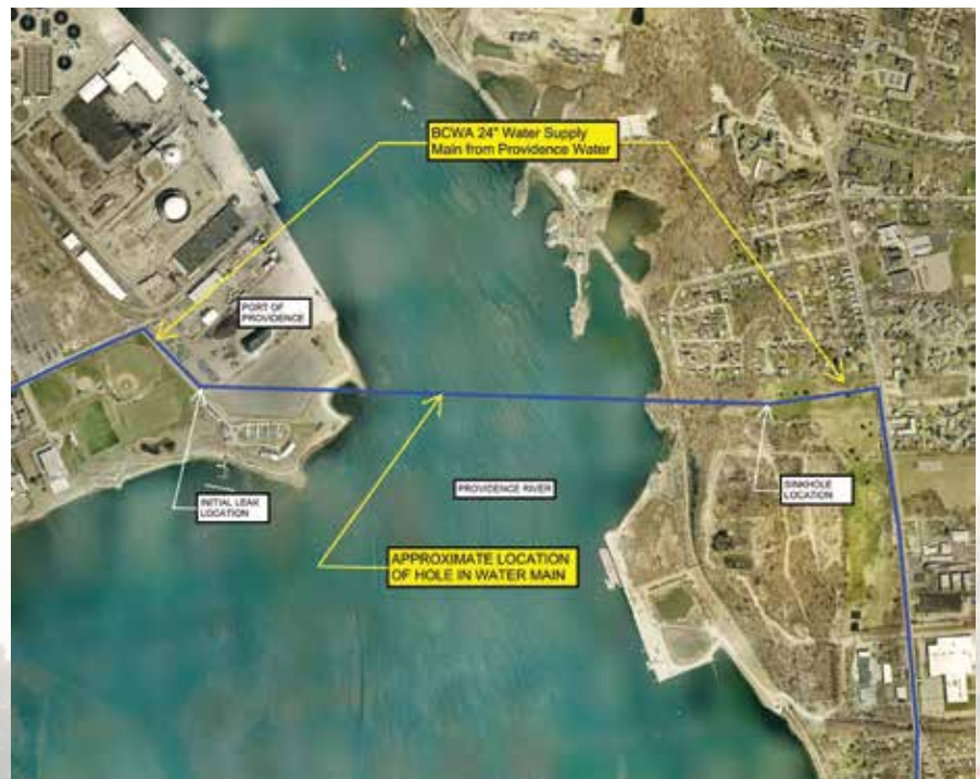
Critical 4,300-foot 24-inch welded steel main crossing under the Providence River originally installed in 1998 by HDD to a depth of approximately 170 feet in bedrock
